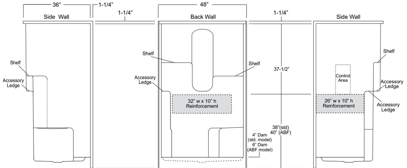
**Package Order No.: 3SM (3-side, mid-level wall reinforcement)**
