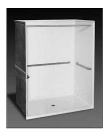
**Specification** – Oasis one-piece FRP gelcoat shower compartment SHFW-6235, having a 60 x 30-inch minimum clear interior dimension and  $\frac{1}{2}$ -inch high maximum finished threshold with floor attachment flange on lower threshold. A factory-equipped package, in compliance with 2010 ADA Standards & ICC/ANSI A117.1-2009 for Accessible Design, shall include a horizontal bar across each side wall and back wall and shower curtain rod.
