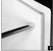
Grab Bars: Factory-installed 1.50-inch diameter, concealed attachment, 18 gauge, #304 brushed stainless steel grab bars. Concealed Photo 1: attachment design provides tamper-resistance and minimizes debris collection areas at contact points, compared to common exposed flange bar designs, without compromising bar attachment integrity. (Reinforced areas include a structural core material encapsulated in FRP composite.)
