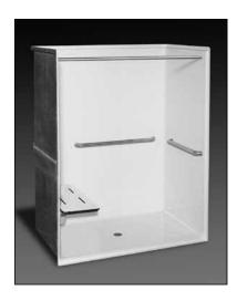
**Specification** – Oasis one-piece FRP gelcoat shower compartment SHFW-6235, having a 60 x 30-inch minimum clear interior dimension and ½-inch high maximum finished threshold with floor attachment flange on lower threshold. A factory-equipped package, in compliance with 2010 ADA Standards & ICC/ANSI A117.1-2009 for Accessible Design, shall include a horizontal bar across the side wall opposite the seat wall and back wall, a folding seat, and shower curtain rod.
