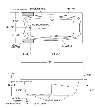
Geneva 3672: TR-B-270 / TRG-270Sump Dimen:59-1/2" long x 26-1/2" wide x 19" deepSump Capacity:70 gal. (unoccupied - to overflow)Whirlpool Operating:35 gal.
