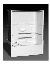
**Specification** – Oasis 3-piece, 60 x 30-inch deep, FRP gelcoat bathtub model TS3P-6030 ABF (17.25-inch apron) having a factory-equipped package in compliance with 2010 ADA Standards for Accessible Design. Package includes 2-horizontal bars on back wall, single horizontal bar on head end wall, horizontal bar on control wall, pivothinge FOLDING in-tub seat at head end and shower curtain rod.
