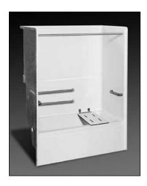
**Specification** – Oasis one-piece, 60 x 32-inch deep, FRP gelcoat flat wall bathtub model TSFW-6032 ABF (18.25-inch apron) having a factory-equipped package in compliance with 2010 ADA Standards for Accessible Design. Package includes 2-horizontal bars on back wall, single horizontal bar on head end wall, horizontal bar on control wall, pivot-hinge FOLDING in-tub seat at head end and shower curtain rod.
