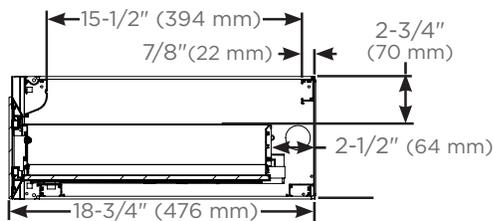
Side views for plumbing and sink clearance with door front
