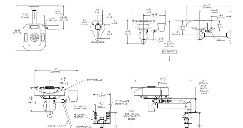
1. All dimensions are in inches (millimeters) unless otherwise specified and are subject to change without notice. 2. This unit should be connected to an uninterrupted source of potable water, with a minimum flowing pressure of 30 psi and a maximum static pressure of 125 psi. 3. Before mounting mixing valve, verify the supply hose will reach the connection.
