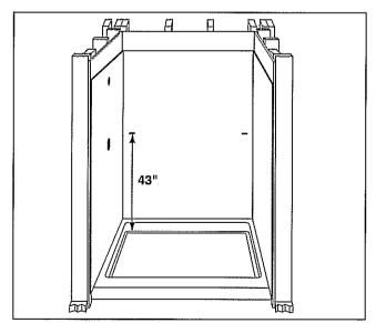
After marking the height, draw a 4" level-line on both walls. These lines will be used to align the top edges of the soap dish.
